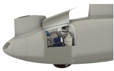
Figure 6.24: Engine bay inspection doors
