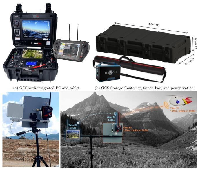
(c) Long range video and telemetry using repeaters and high-gain parabolic antennas
