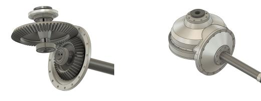
(b) Bevel gear meshing
