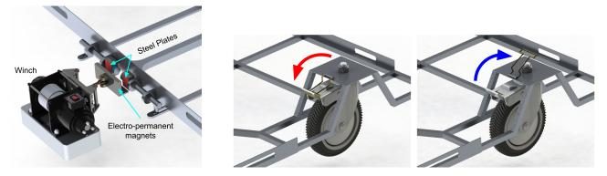
Figure 6.16: Electromagnetic Release
