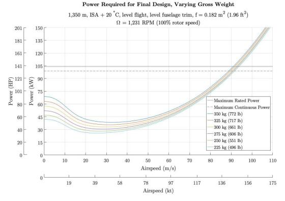
Figure 12.4: Level flight performance, varying gross weight
